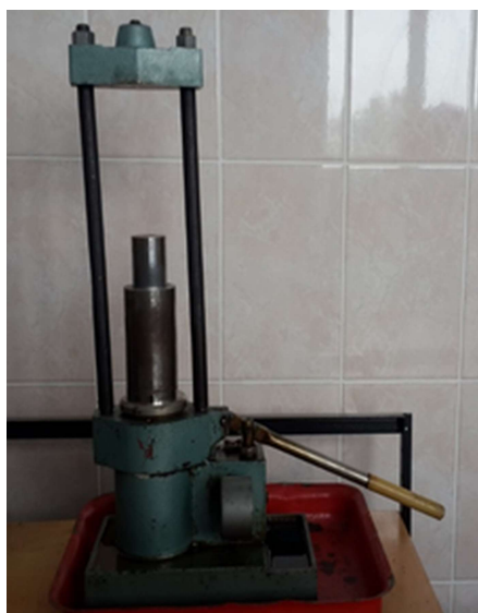
Fig. 2 The compression mold and the stamp press.
