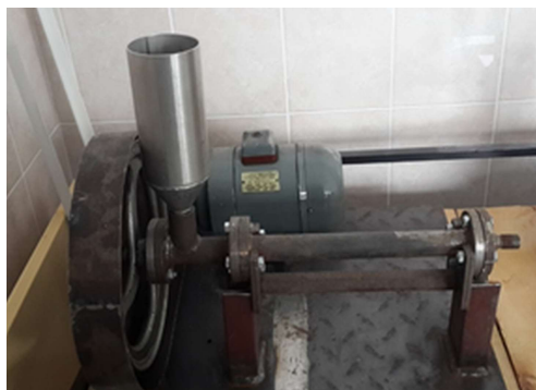
Fig. 1 The extruder-type mixing machine design.
