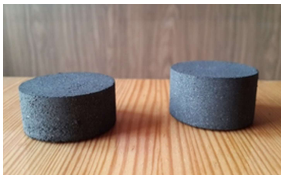
Fig. 3 Coal and coke dust briquettes with a substandard urea binder.
