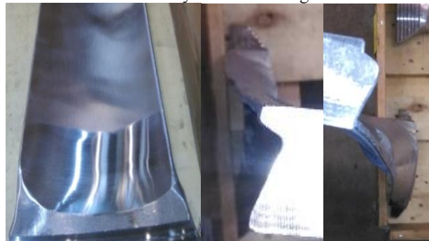
Fig. 3. Poor condition of a new oOEM LSB used for reverse engineering.
