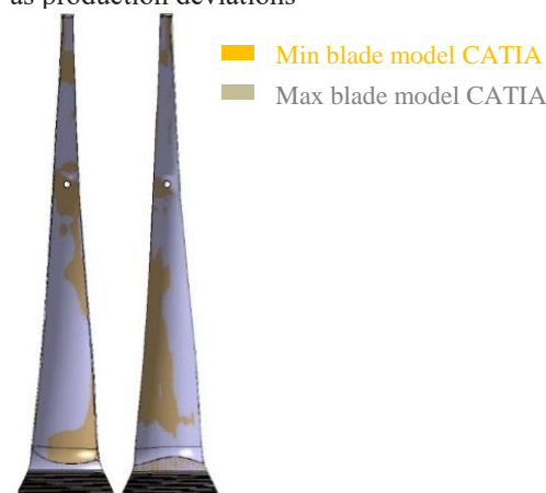
Fig. 4. Comparison of min, max models CATIA.
