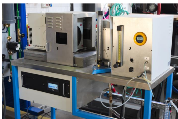
Fig. 1. Experimental setup scheme (upper) and actual photo (lower) of the research stand: 1, xenon arc lamp, 2, insulated reactor, 3, PLC and measurements devices container, 4, lamp power supply, 5, bio-oil condenser.
