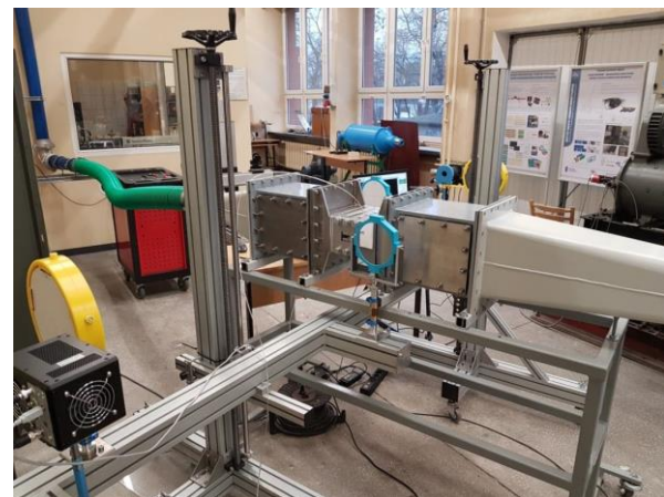
Fig. 5 Test section with schlieren apparatus.
