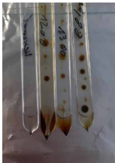
Figure 2c: Ferrofluids after condensation at room temperature at 1 w% in capillaries.
