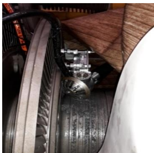
Fig. 2. Specimen sampling from a 200 MW turbine rotor disc
