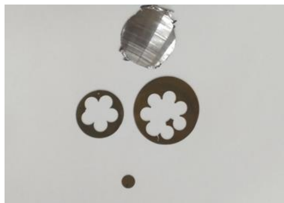
Fig. 3. Rotor material specimen and the micro specimens made of it
