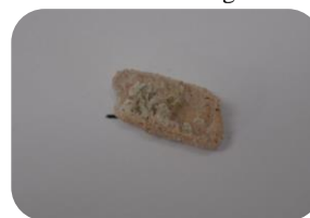
Fig 6. Residue after combusting sunflower husk pellets at 850°C and G_s = 5 \text{ kg/m}^2\text{s} .
