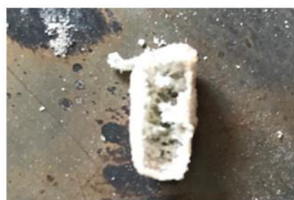
Fig 6. Residue after combusting sunflower husk pellets at 850°C and G_s = 5\text{kg/m}^2\text{s} .
