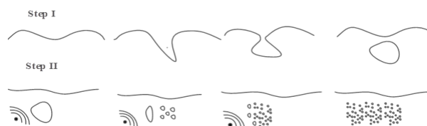
Fig. 2. Ultrasound emulsification: droplet formation and breakup.
