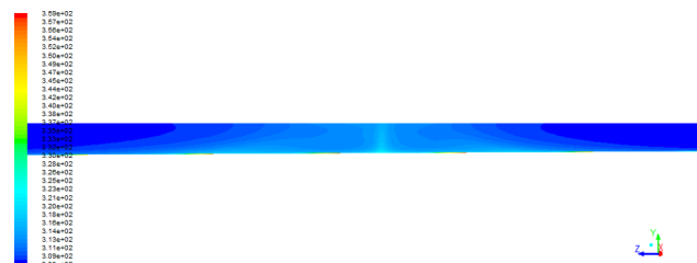
Fig.8. Central Longitudinal Section Temperature Cloud Diagram II inside the noise barrier Unit: K
