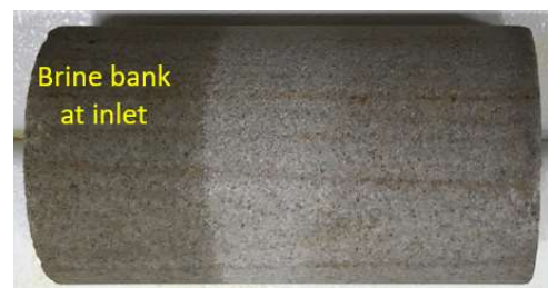
Fig. 1. Berea sandstone sample taken from test rig at the early stage of an imbibition Rel Perm measurement using standard, co-current SCAL methods. A large brine bank has formed at the inlet that blocks the permeability to gas.
