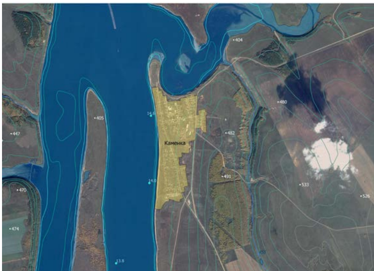
Fig. 5. A fragment of the resulting map for the Bratsk reservoir near the Kamenka settlement. The bathymetry contour lines were obtained from pilot charts.
