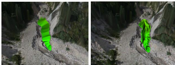
Fig. 3. 3D image of a DTM fragment, with a surface along the ground points of the embankment contour and a height file with the selected embankment surface.
