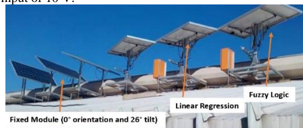
Fig. 2. The practical system with the PV modules highlighted.
