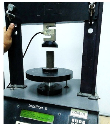
Fig.4. The unconfined compressive strength test machine
