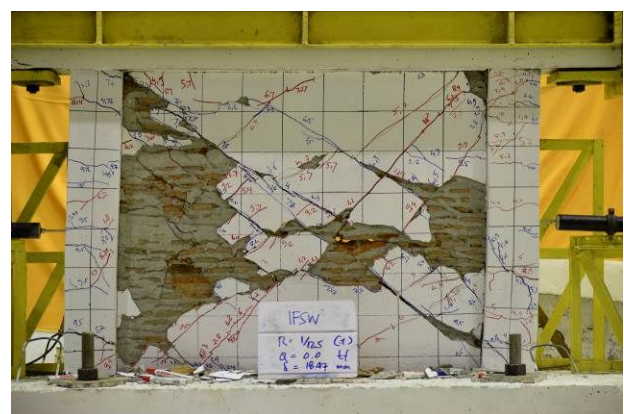
(b) Crack Pattern at R=+1/12.5
