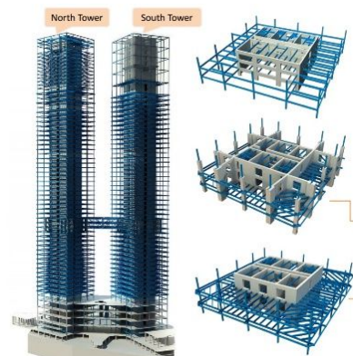
Fig 2. Structural System of Indonesia-1
