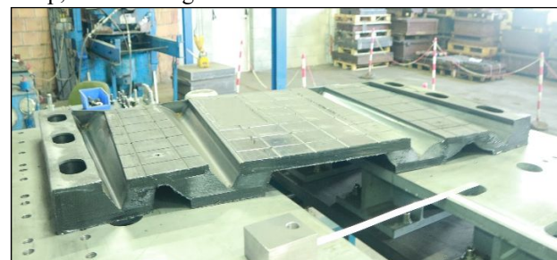
Fig. 7. Documentation from Seismic SFX Joint Test (Simultaneous movement of Long – Trans)
