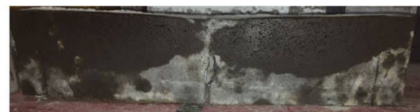
Fig. 12 SRPC Specimen After Being Subjected to Single Notch TPB Test
