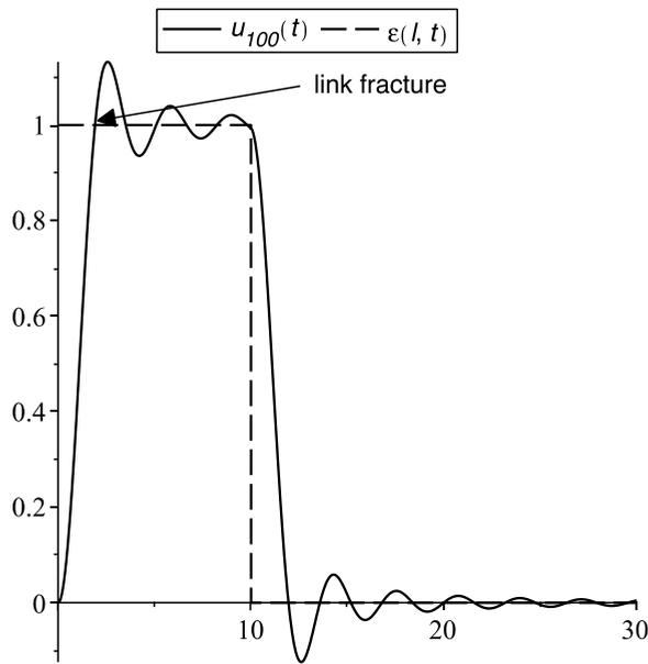
**Fig. 5.** Deformation of the chain link with number  $N$  (solid line) and rod deformation at point  $x = l$  (dashed line). Link fracture is indicated by an arrow. In this case number of links  $N = 100$  and rod length  $l = 100$ .
