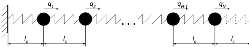
**Fig. 1.** Uniformly deformed chain with an abruptly failing link.
