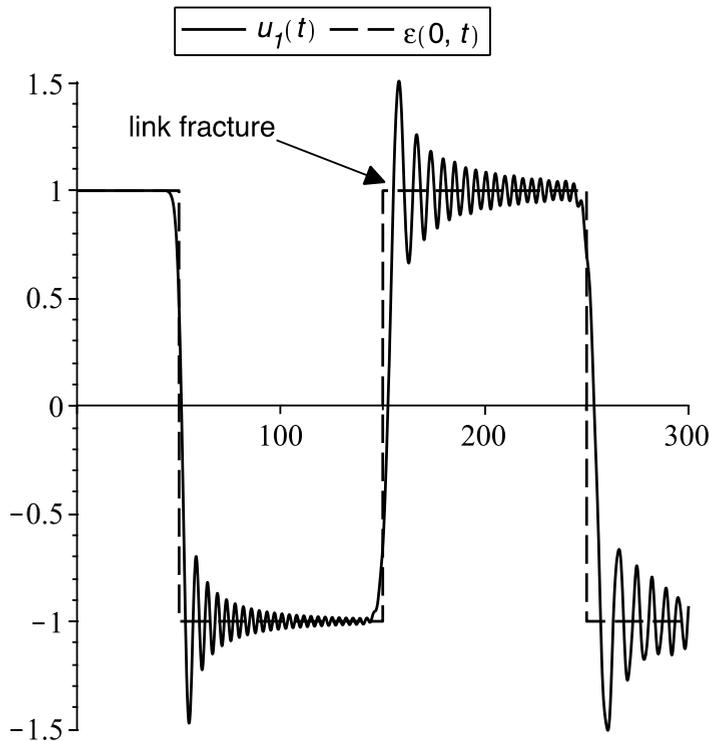
**Fig. 4.** Deformation of the first chain link (solid line) and deformation of rod in a sealed point (dashed line). Arrow indicates the link fracture. Results for 50 links and a rod with length  $l = 50$  are shown.
