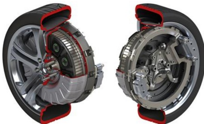
Fig. 2. Power units of electric vehicles with one electric motor per wheel
