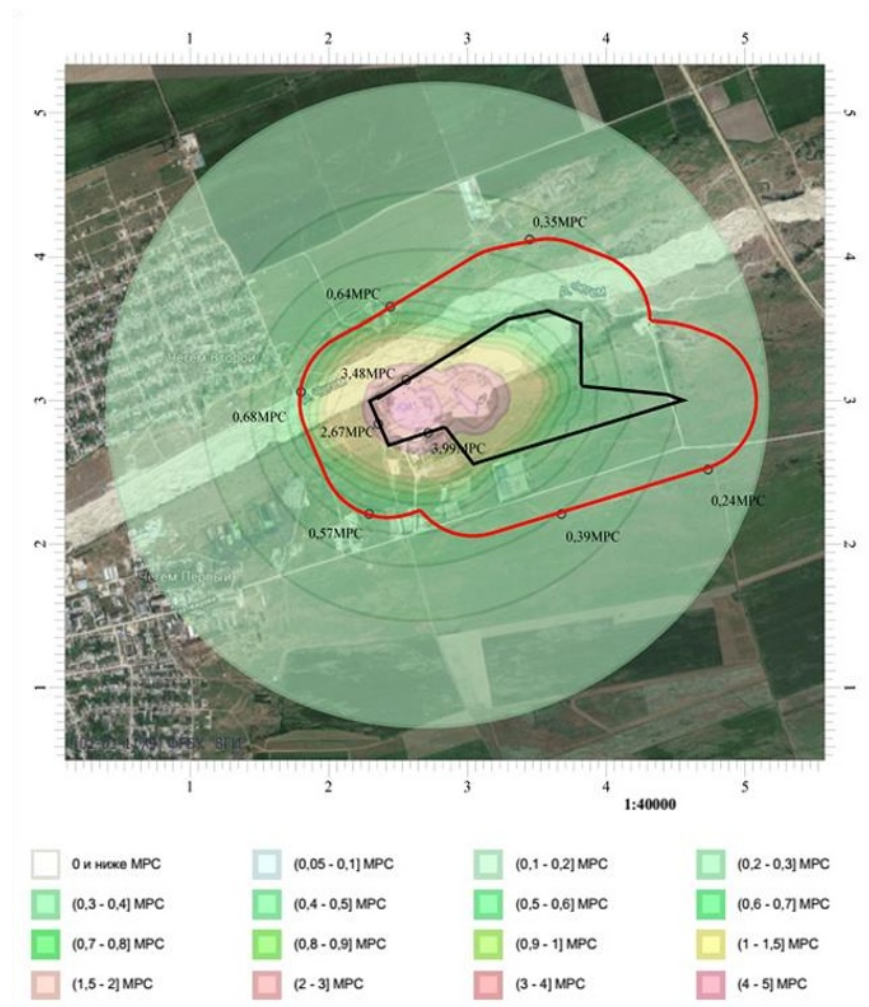
Fig.1. Inorganic dust dispersion map in the area of the enterprise location: the red polygon is the boundary of the sanitary protection zone, the black polygon is the boundary of the enterprise
