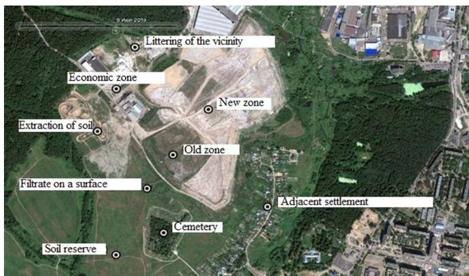
Fig. 1: Main components of WDF on the example of solid household waste landfill (SHW) "Kuchino"
