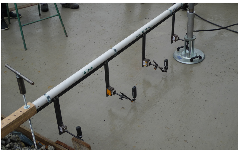
Fig. 4. Measurement apparatus for PLT testing.
