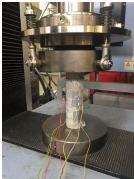
Fig. 5. Compression test of the core sample
