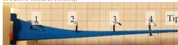
Figure 3. 3D printed blade subjected to the test stand
