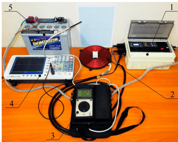
Fig. 2. Laboratory stand for measuring the distribution of pulsed magnetic induction: 1 – automated MPP device, 2 – magnetic inductor, 3 – milliteslameter portable universal (TPU-01), 4 – digital oscilloscope AKIP 4122/1, 5 – battery.
