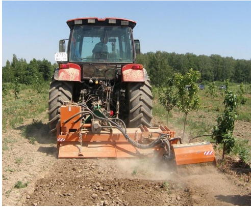
Fig. 7. Model of a garden cutter with a remote milling section in operation.
