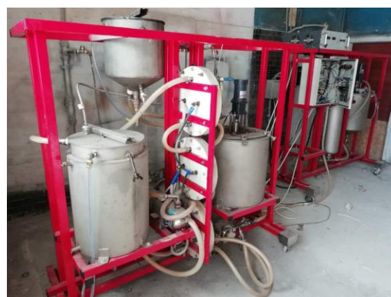
Fig. 2. The experimental electrochemical installation for producing protein hydrolyzate from SRM.
