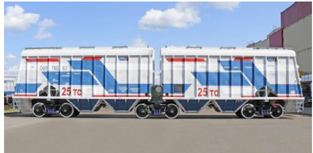
Fig. 3. An articulated hopper car.
