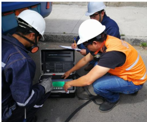
Fig. 2. GHG Bachacach ECA 450 measuring equipment.
