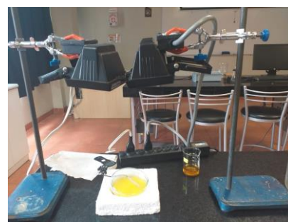
Fig. 2. Evaluation of the temperature gradient of the heat transfer fluids by direct radiation to the study solution.
