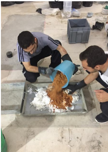
Fig. 4. Mixing of Concrete Ingredients
