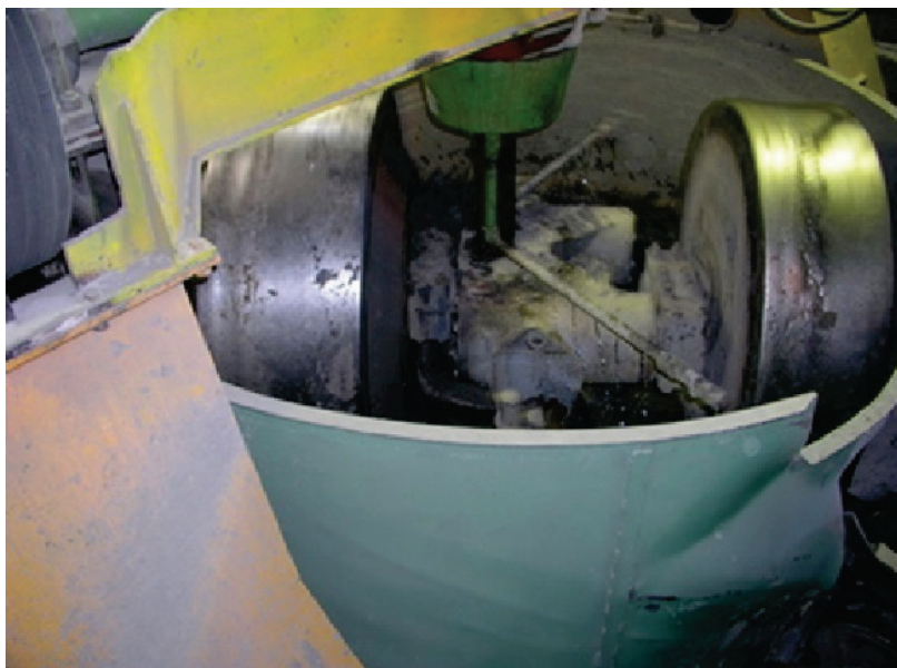
Fig. 8. Wheel mill, Source: M. Vavro 2004.
