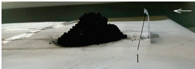
Fig. 4. Coal pile model: 1 – barrier (scenario #2).
