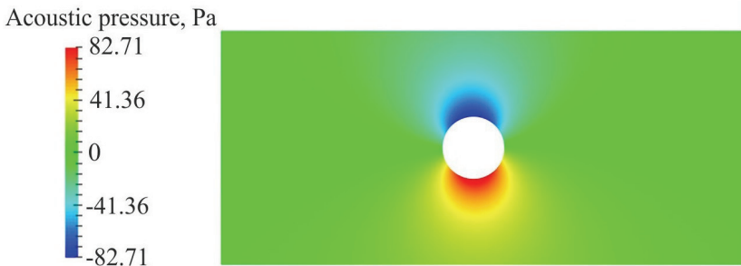
Fig. 4. Distribution of instantaneous acoustic pressure, calculated using the Curle analogy in the flow around a standalone circular cylinder.
