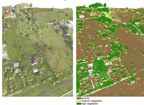
Fig. 2. LIDAR data visualisation a) RGB colour, b) point classification
