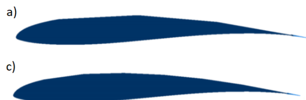
Fig. 2. Shapes of modified airfoils with a) 3, b) 6 flat surfaces.
