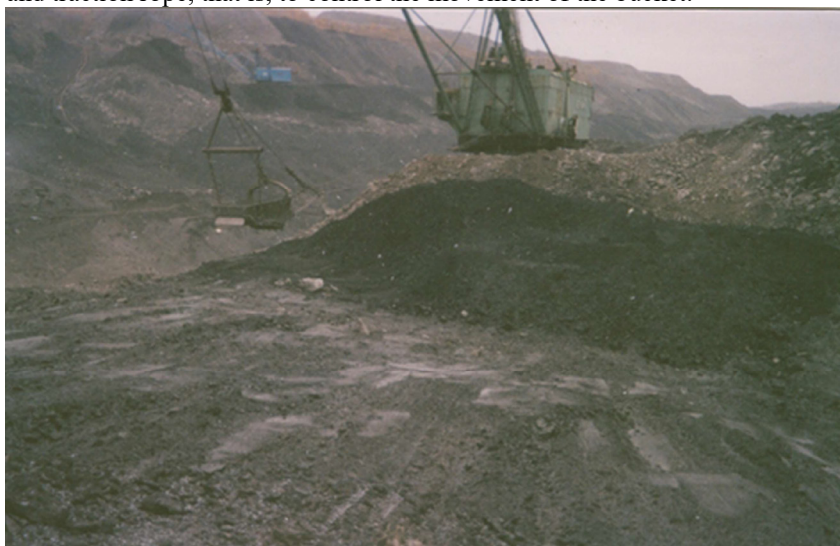
Fig. 3. Filling the bucket of the dragline ESh10.70 with coal during the development of the Volkovsky layer at the Chernigov section, the Chernihiv field.
