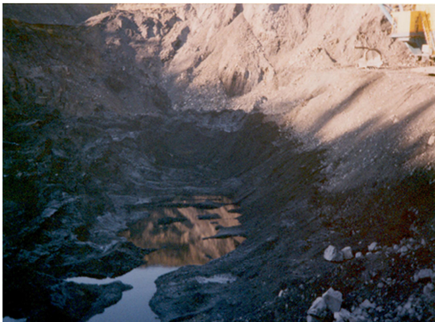
Fig. 2. Type of coal mining face when developing with dragline ESh10.70 in the Kedrovsky open pit (Northern Kuzbass) – the section of the Latsyshevsky site.
