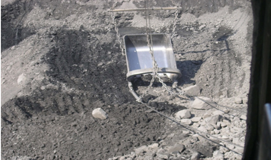
Fig. 1. Scraping the roof of the seam with dragline ESh10.70 at the Sartaki open pit, Central Kuzbass.
