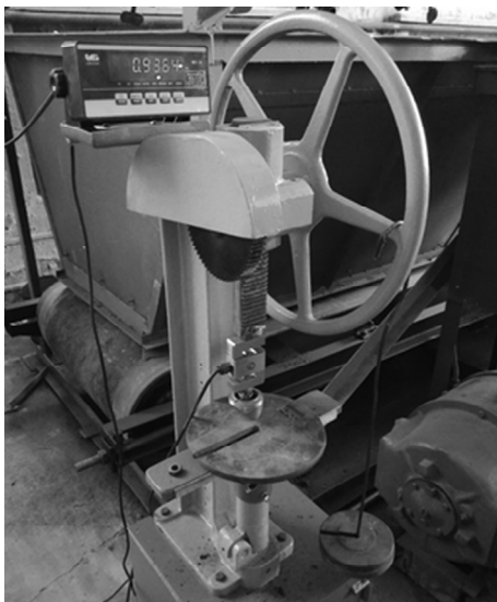
Fig. 2. The process of strain-gauge bracket calibration with calibrated weights.
