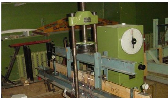
Fig. 2. Test rig with reinforced wooden beam B-2.
