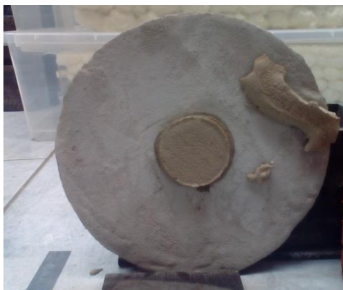
Fig. 1. Estimation of runoff of a clay-gypsum mixture reinforced with fiber from a concrete base.
