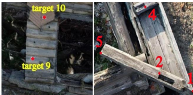
Fig. 4. Fragment of a 3D model with several wall markers and characteristic points involved in measurements.
