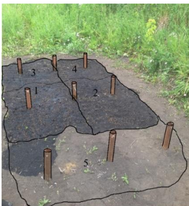
Fig. 1. Type of pollution zone and electrochemical treatment zone: 1 - array contaminated with waste oil; 2 - an array contaminated with gasoline; 3 - array contaminated with waste oil treated with a solvent; 4 - array contaminated with gasoline with solvent treatment; 5 - pure clay massif
