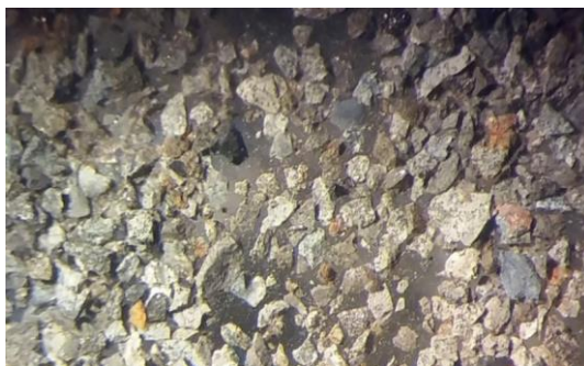
Fig. 6. Fine intergrowth of metallic and nonmetallic phases, brown films of ferrum hydroxides. Zooming 75.
