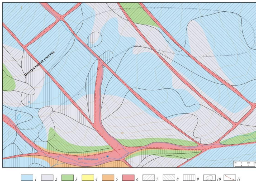
Fig. 3. Fragment of permafrost distribution map of Sofronovskoye deposit
