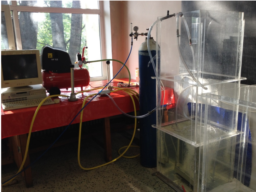
Fig. 7. Overview of the experimental installation for the introduction of a mixture (air + oxygen).
