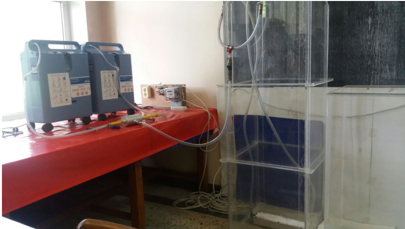
Fig. 9. Overview of the experimental installation for low nitrogen content air supply [5].
