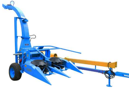
Fig. 1. Trailed Miscanthus stalk harvester - CRM1.6
