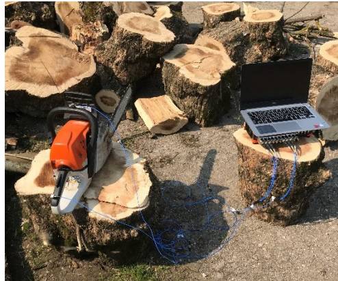
Fig. 1 Test setup for vibration measurement.
