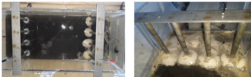
Fig. 8. Intense foaming at the anode during testing
